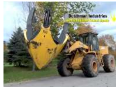
[8] After the tree is raised vertically from the ground the tree is tilted into a horizontal position. The stabilizers are raised and the tree is ready for transporting to its new location.
