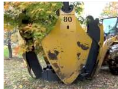
[4] The gate is closed and locked hydraulically.
