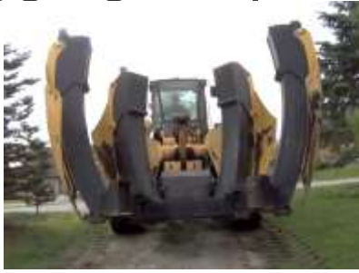
[1] The tree spade is positioned up-right with the blades raised and the gate open.
