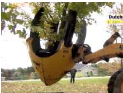
[7] The spoon shaped blades follow a curvilinear track forming a totally enclosed pod of roots and soil.
